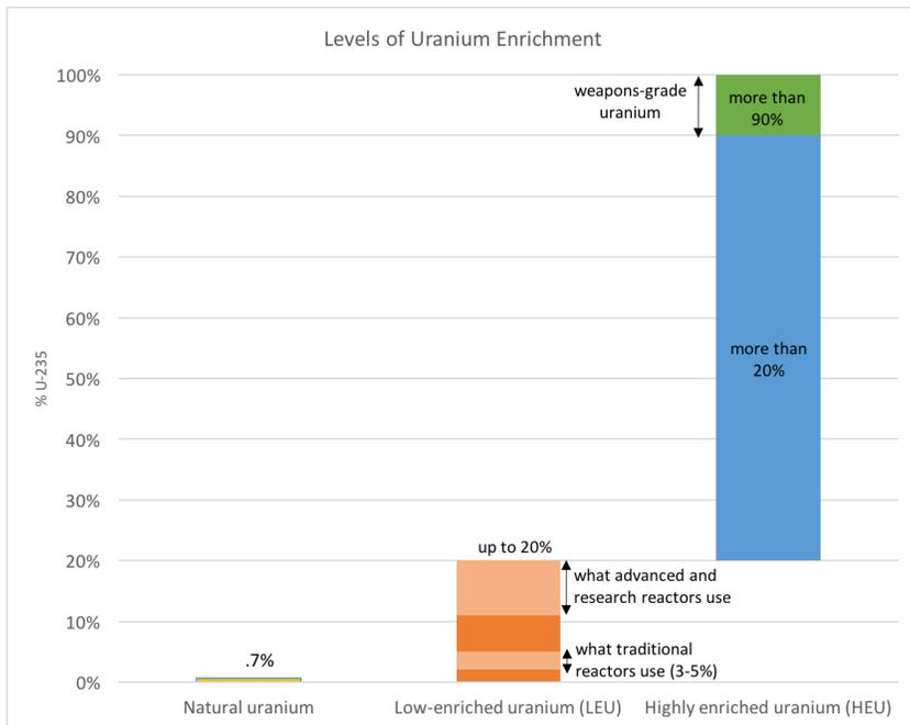
Naturally occurring uranium harvested from mines only has a concentration of 0.7% U-235 isotope. However, this concentration is not high enough for nuclear reactions to occur. Nuclear reactors require “enriched” uranium, meaning the U-235 needs to be further concentrated. Uranium is enriched to different levels, depending on its end-use.
